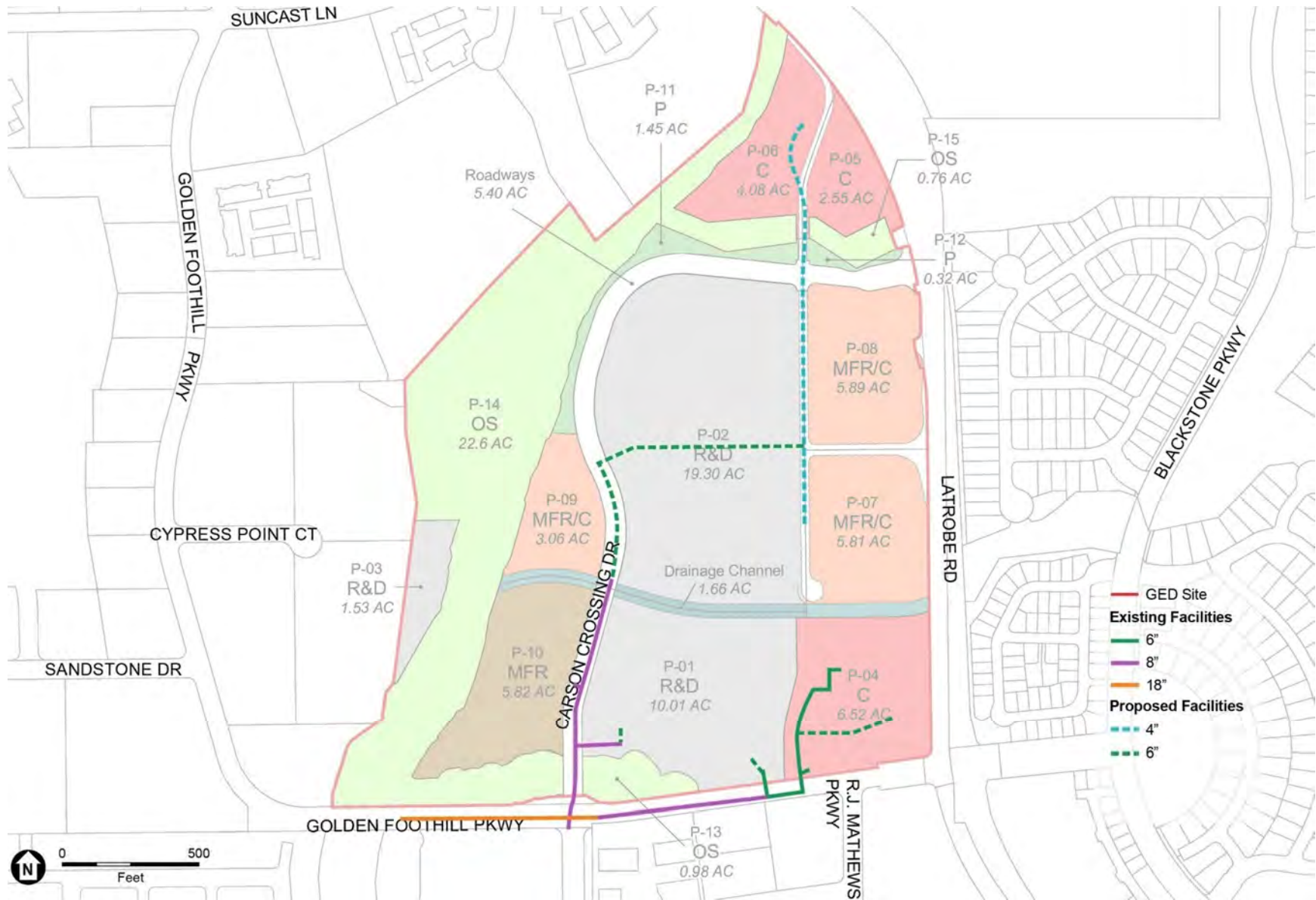
Figure 4.12: GED Backbone Wastewater Collection System
