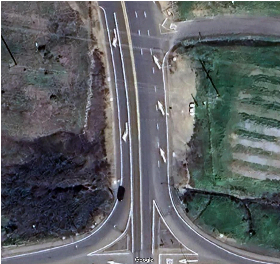
Westbound Bass Lake Road-US50 Interchange offramp lane striping - merge arrows point to one lane that becomes two lanes, that becomes one lane.
