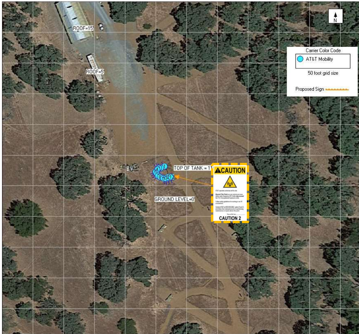
Figure 2: Mitigation Recommendations Caution 2 sign required on the base of the Faux Water Tank at the access location
