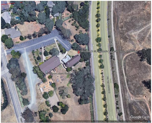
The Second Collocation that was investigaged was the St. Stephen's Lutheran Church where T-Mobile has a stealthed faclity. After further research, there is no additional space within the T-Mobile Stealthed Facility. Furthermore, installing a free-standing structure was not an option due to restrictive CC&R's that does not allow such free-standing structures but only attached structures to the church. For these reasons, this candidate was disqualified as a viable candidate.
