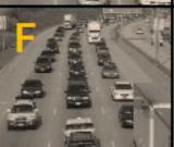
Forced or breakdown conditions. Exists wherever the volume of traffic exceeds the capacity of the roadway.
