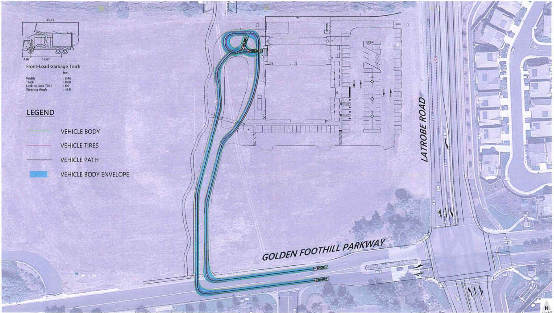
Figure 3 El Dorado Hills Tractor Supply Company Truck Turning Exhibit Front-Load Garbage Truck
