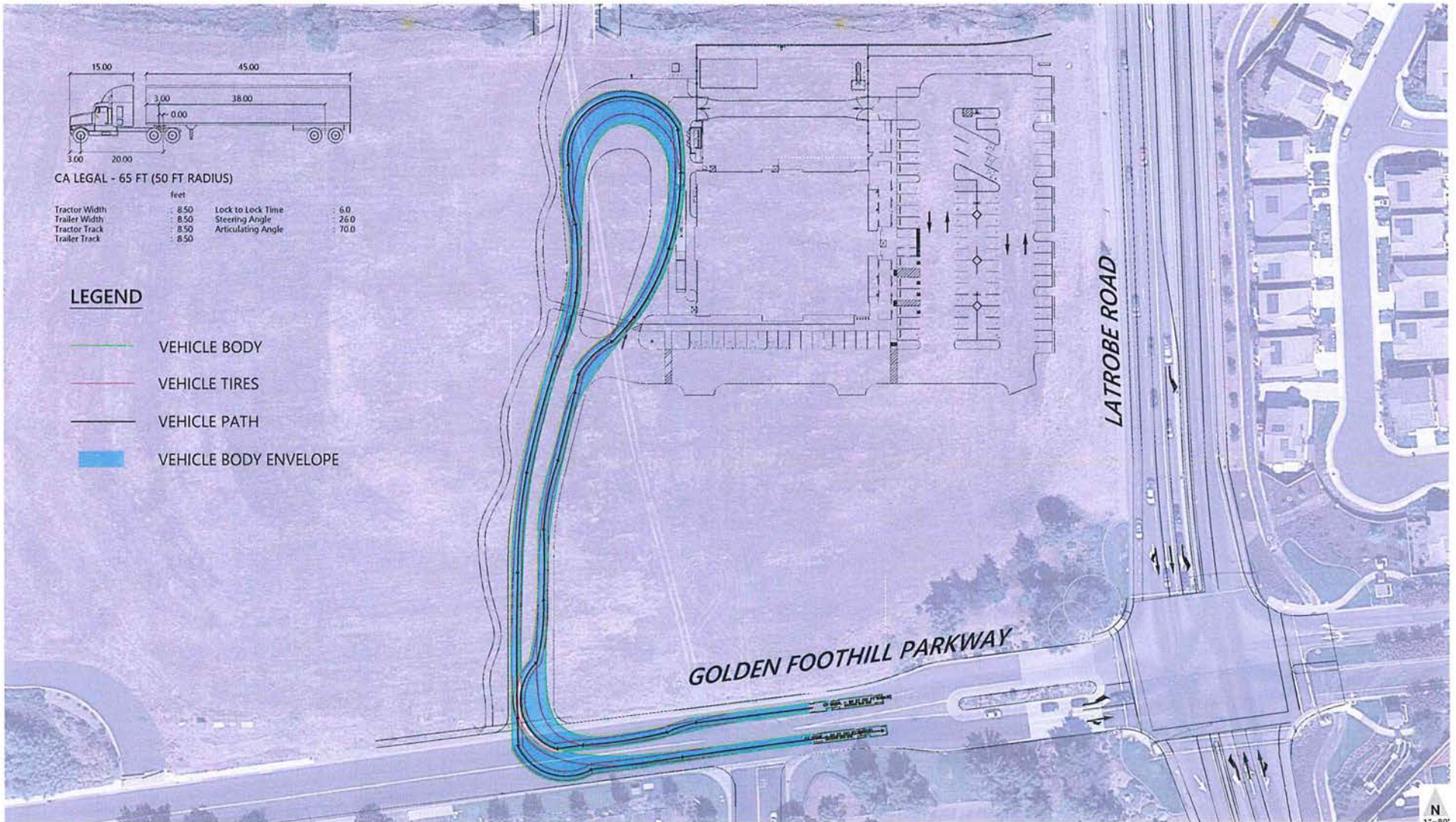
Figure 1 El Dorado Hills Tractor Supply Company Truck Turning Exhibit CA Legal - 65 Ft
